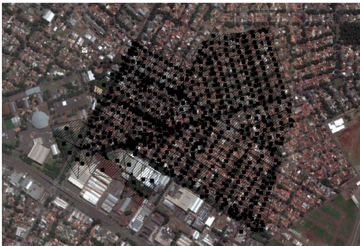
Fig 2. Detail of the definition of drainage sub-basins, catchbasins and conduits in the EPA SWMM program.
